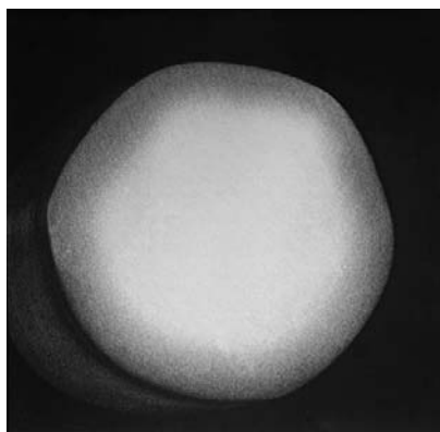
Fig. 1. Cross section of sapphire fiber with a Ti-doped central part, grown by the modified Stepanov method with a specified radial gradient of composition and optical properties.
