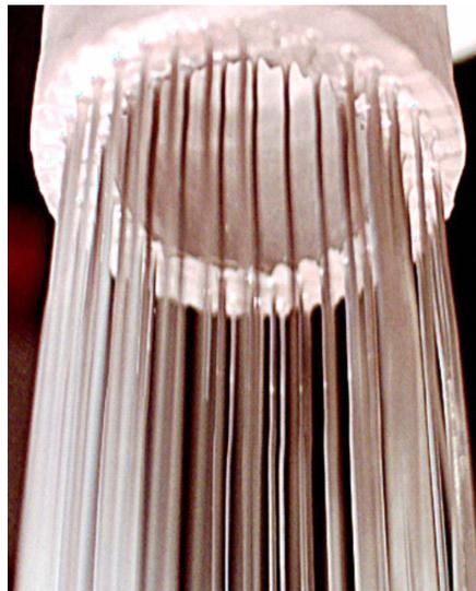
**Fig. 5** Sapphire fibers of 250-300  $\mu\text{m}$  in diameter grown by multi – run crystal growth process. (Online color at [www.crt-journal.org](http://www.crt-journal.org))
