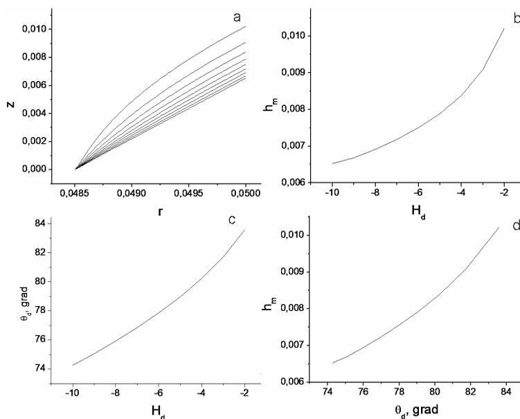
**Fig. 2** a – profile curves of the small internal menisci (capillaries) for the various values of the external pressure, b – dependence of the meniscus height on the external pressure, c – dependence of the angle  $\theta_d$  on the external pressure, d – dependence of the meniscus height on the angle  $\theta_d$  at various values of the external pressure.
