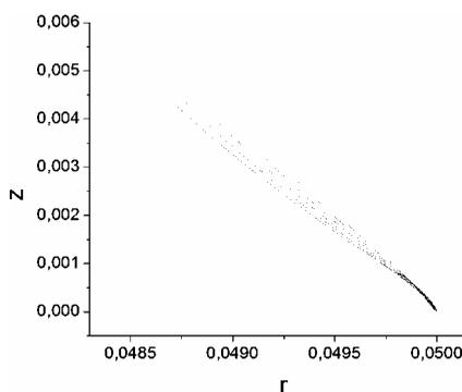
**Fig. 3** Profile curves of the small external menisci (fibers) at the various values of the crystal radius. Case of negative angles  $\theta_d$ .
