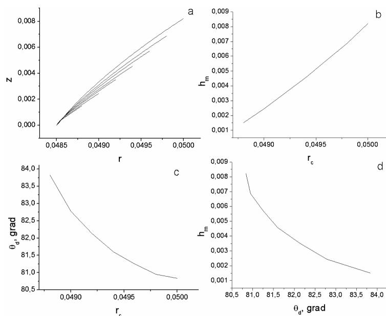
**Fig. 1** a – profile curves of the small internal menisci (capillaries) at the various values of the crystal radius, b – dependence of the meniscus height on crystal radius, c – dependence of the angle  $\theta_d$  on the crystal radius, d – dependence of the meniscus height on the angle  $\theta_d$ . Case of the positive angles  $\theta_d$ .
