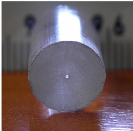
**Fig. 4** Sapphire rod of 10 mm in external diameter with capillary channel of 450  $\mu\text{m}$ . (Online color at [www.crt-journal.org](http://www.crt-journal.org))
