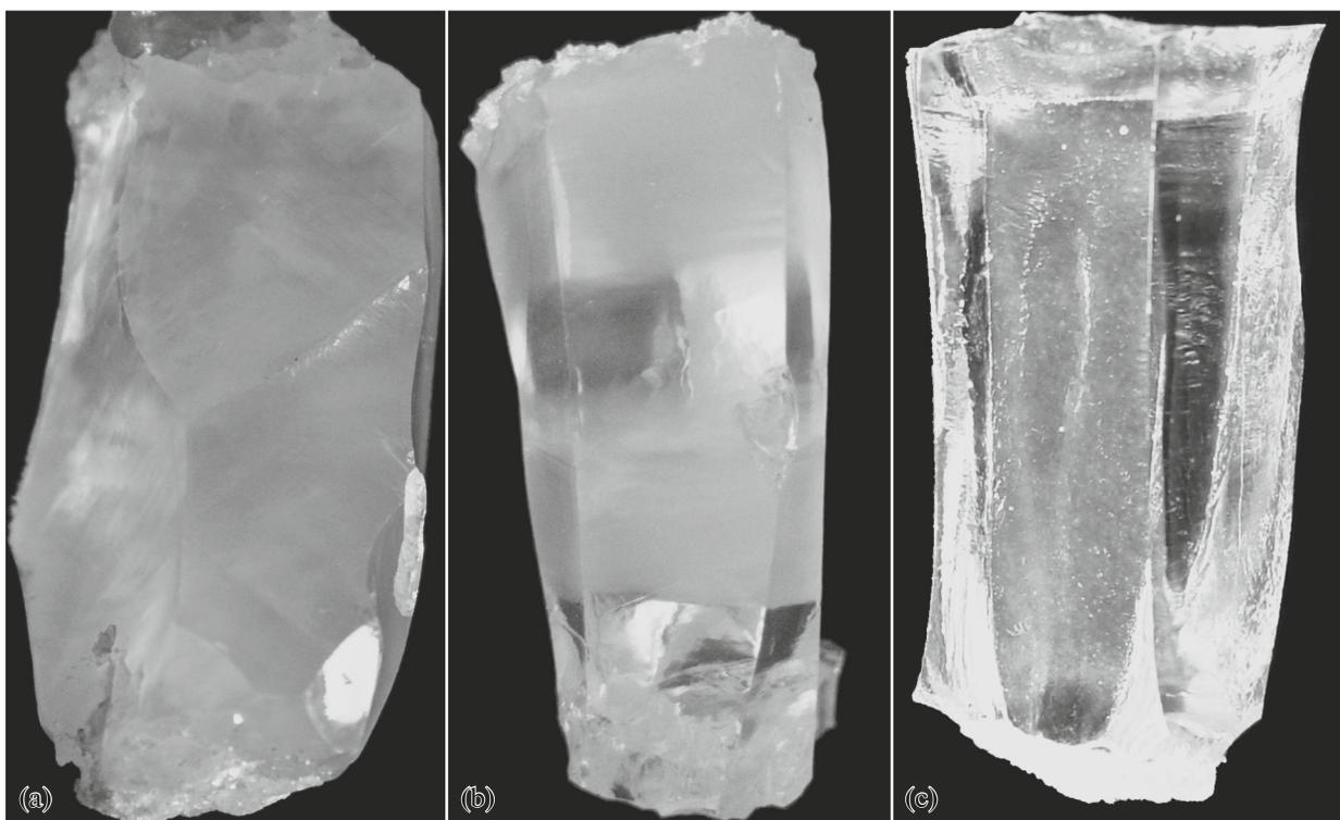
**Fig. 1.** View of the crystals: (a) semi-transparent, (c) transparent, and (b) with alternating transparent and semi-transparent regions.
