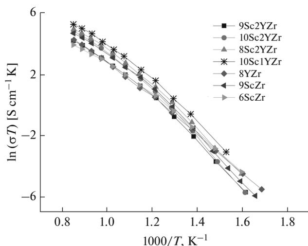
**Fig. 5.** Temperature dependences of specific conductivity of  $(\text{ZrO}_2)_{1-x-y}(\text{Sc}_2\text{O}_3)_x(\text{Y}_2\text{O}_3)_y$  crystals.
