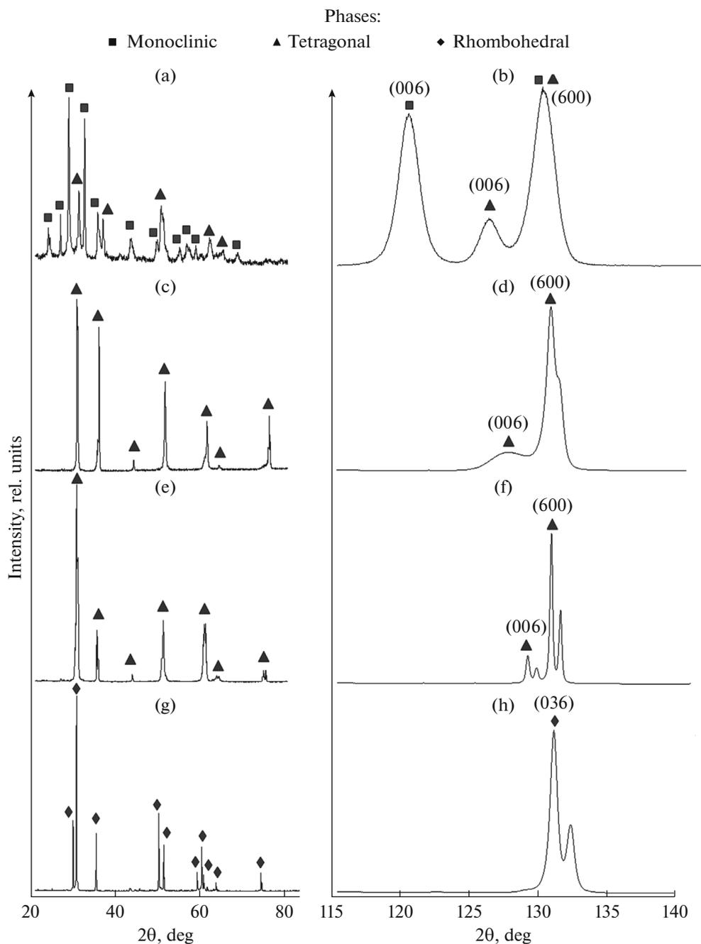
**Fig. 2.** Diffraction patterns of the (a, c, e, g) powder and (b, d, f, h)  $(\text{ZrO}_2)_{1-x}(\text{Sc}_2\text{O}_3)_x$  single-crystal samples: (a, b) 3.5ScZr; (c, d) 6ScZr; (e, f) 9ScZr; and (g, h) 11ScZr.
