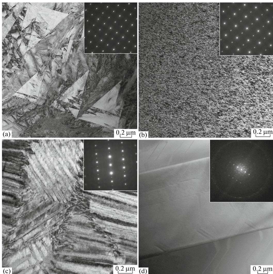
**Fig. 4.** TEM images of  $(\text{ZrO}_2)_{1-x}(\text{Sc}_2\text{O}_3)_x$  crystals: (a) 3.5ScZr, (b) 6ScZr, (c) 9ScZr, and (d) 11ScZr. Inserts: diffraction patterns from the corresponding regions of the crystals.
