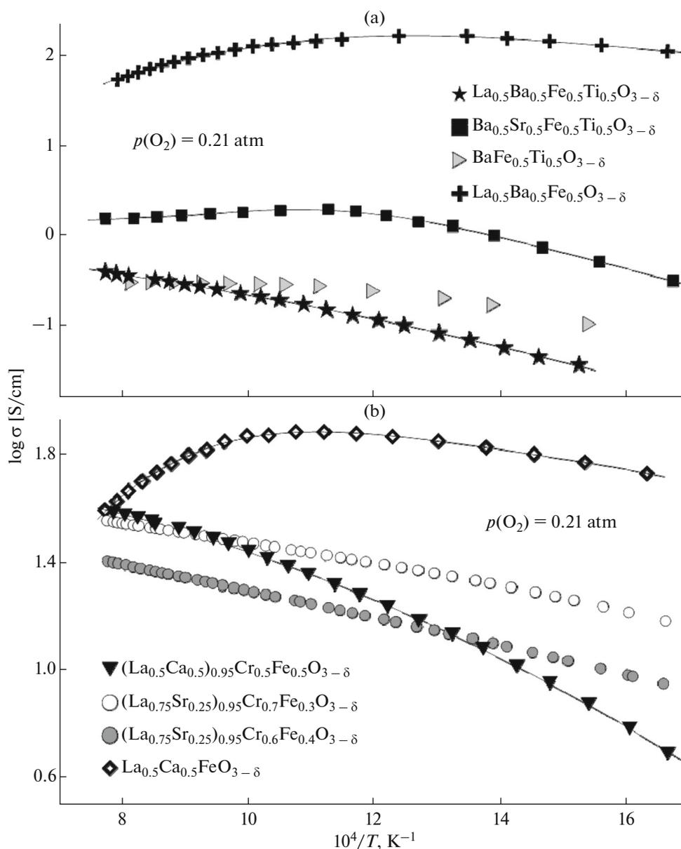
**Fig. 4.** Temperature dependences of the specific conductivity of ceramic samples for (a)  $La_{0.5}Ba_{0.5}Fe_{0.5}Ti_{0.5}O_{3-\delta}$  and (b)  $(La_{0.5}Ca_{0.5})_{0.95}Cr_{0.5}Fe_{0.5}O_{3-\delta}$  in air. For a comparison, the results of [14, 37] are shown.
