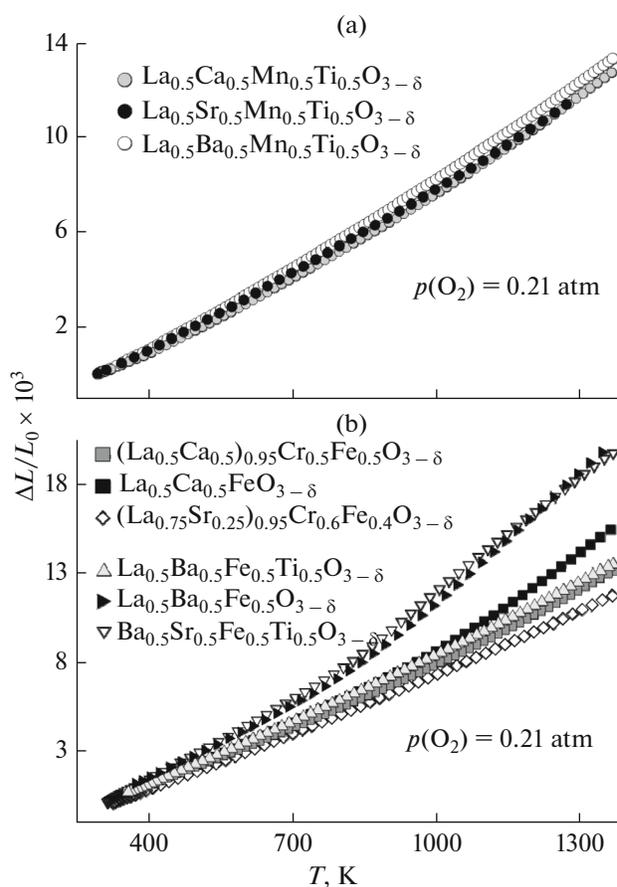
**Fig. 6.** Dilatometric curves measured in air for (a)  $\text{La}_{0.5}\text{A}_{0.5}\text{Mn}_{0.5}\text{Ti}_{0.5}\text{O}_{3-\delta}$  ( $A = \text{Ca}, \text{Ba}$ ) and also for (b)  $\text{La}_{0.5}\text{Ba}_{0.5}\text{Fe}_{0.5}\text{Ti}_{0.5}\text{O}_{3-\delta}$  and  $(\text{La}_{0.5}\text{Ca}_{0.5})_{0.95}\text{Cr}_{0.5}\text{Fe}_{0.5}\text{O}_{3-\delta}$  in the mode of permanent cooling at a rate of 3 K/min. For a comparison, the results of [14, 22, 37] are shown.
