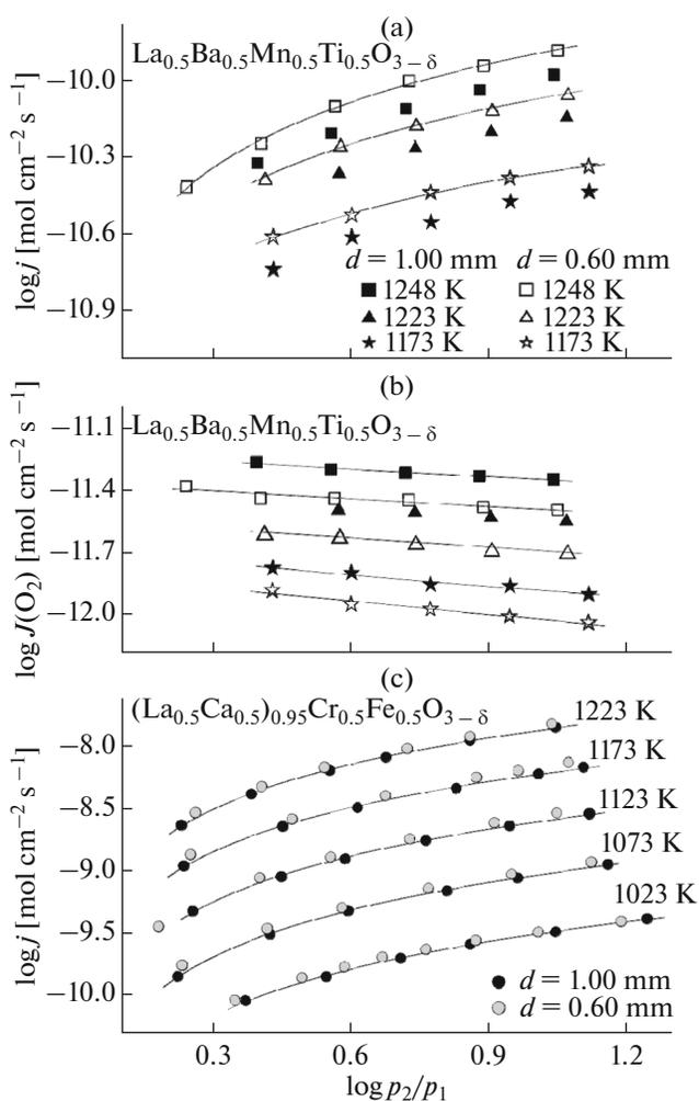
**Fig. 9.** Isothermal dependences of (a, c) specific oxygen flow and (b) specific oxygen permeability through gas-tight membranes of (a, b)  $\text{La}_{0.5}\text{Ba}_{0.5}\text{Mn}_{0.5}\text{Ti}_{0.5}\text{O}_{3-\delta}$  and (c)  $(\text{La}_{0.5}\text{Ca}_{0.5})_{0.95}\text{Cr}_{0.5}\text{Fe}_{0.5}\text{O}_{3-\delta}$  with the thickness of 1.00 mm and 0.60 mm. The partial oxygen pressure on the fed side of the membrane ( $p_2$ ) is 0.21 atm.
