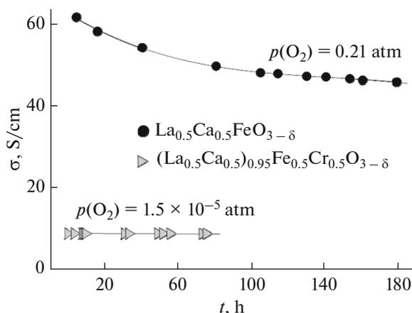
**Fig. 5.** Time dependences of the specific conductivity for  $(\text{La}_{0.5}\text{Ca}_{0.5})_{0.95}\text{Cr}_{0.5}\text{Fe}_{0.5}\text{O}_{3-\delta}$  ( $p(\text{O}_2) = 1.5 \times 10^{-5} \text{ atm}$ ) and  $\text{La}_{0.5}\text{Ca}_{0.5}\text{FeO}_{3-\delta}$  ( $p(\text{O}_2) = 0.21 \text{ atm}$ ) at 1223 K.
