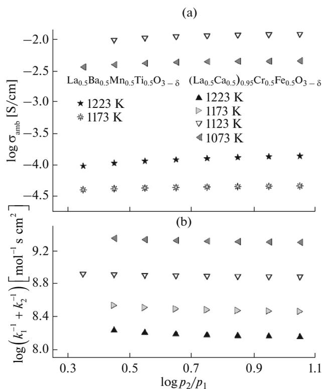
**Fig. 10.** Isothermal dependences of (a) conductivity and (b) the sum of reciprocal constants of surface exchange found within the framework of a model described in [41] on the drop of partial oxygen pressure for ceramic membranes (a)  $\text{La}_{0.5}\text{Ba}_{0.5}\text{Mn}_{0.5}\text{Ti}_{0.5}\text{O}_{3-\delta}$  and (a, b)  $(\text{La}_{0.5}\text{Ca}_{0.5})_{0.95}\text{Cr}_{0.5}\text{Fe}_{0.5}\text{O}_{3-\delta}$ .
