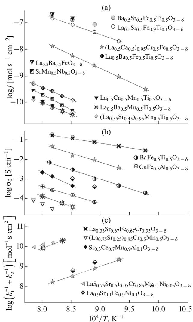
**Fig. 8.** (a) Temperature dependences of the specific oxygen flow through gas-tight membranes ( $d = 1.00$  mm) at the fixed drop of partial oxygen pressure  $p_2/p_1 = 1.0$ . Temperature dependences of (b) ionic conductivity and (c) the sum of reciprocal constants of surface exchange, calculated in the framework of a model described in [41], at  $p(\text{O}_2) = 0.21$  atm. For a comparison, the results of [8, 22, 27, 41, 60–62] are shown.
