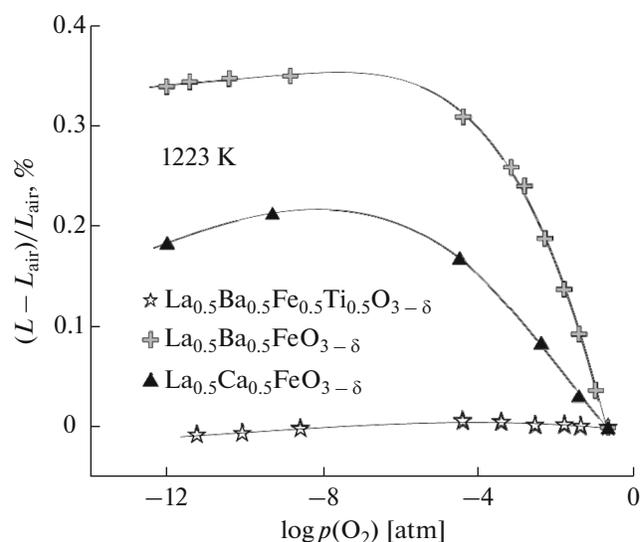
**Fig. 7.** Isothermal dependences of the changes in the length of ceramic samples based on  $\text{La}_{0.5}\text{Ba}_{0.5}\text{Fe}_{0.5}\text{Ti}_{0.5}\text{O}_{3-\delta}$ ,  $\text{La}_{0.5}\text{Ba}_{0.5}\text{FeO}_{3-\delta}$ , and  $\text{La}_{0.5}\text{Ca}_{0.5}\text{FeO}_{3-\delta}$  with respect to their initial length in air on the partial oxygen pressure.
