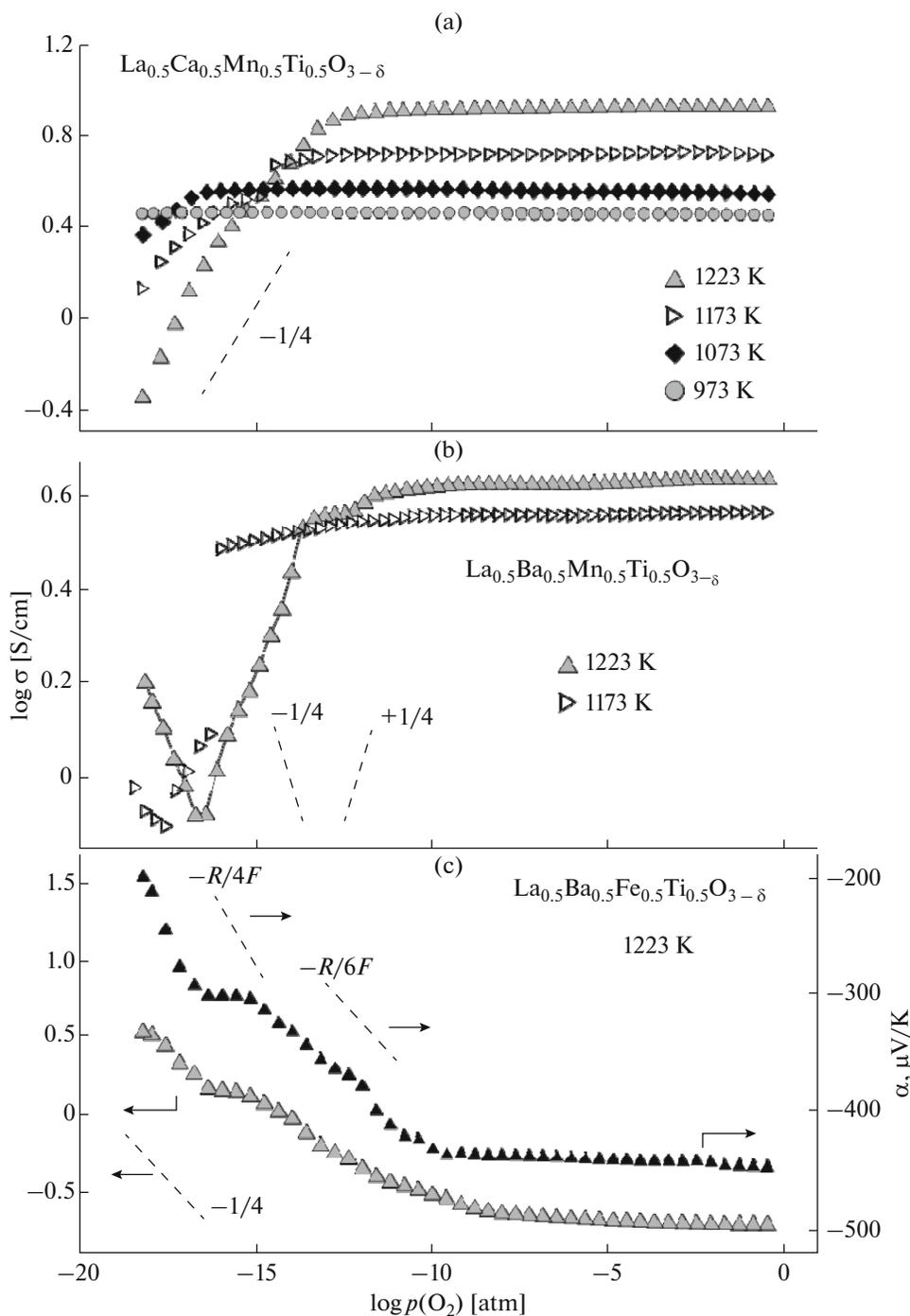
**Fig. 3.** Isotherms of specific conductivity and the Seebeck coefficient for ceramic samples of (a)  $\text{La}_{0.5}\text{Ca}_{0.5}\text{Mn}_{0.5}\text{Ti}_{0.5}\text{O}_{3-\delta}$ , (b)  $\text{La}_{0.5}\text{Ba}_{0.5}\text{Mn}_{0.5}\text{Ti}_{0.5}\text{O}_{3-\delta}$ , (c)  $\text{La}_{0.5}\text{Ba}_{0.5}\text{Fe}_{0.5}\text{Ti}_{0.5}\text{O}_{3-\delta}$ .
