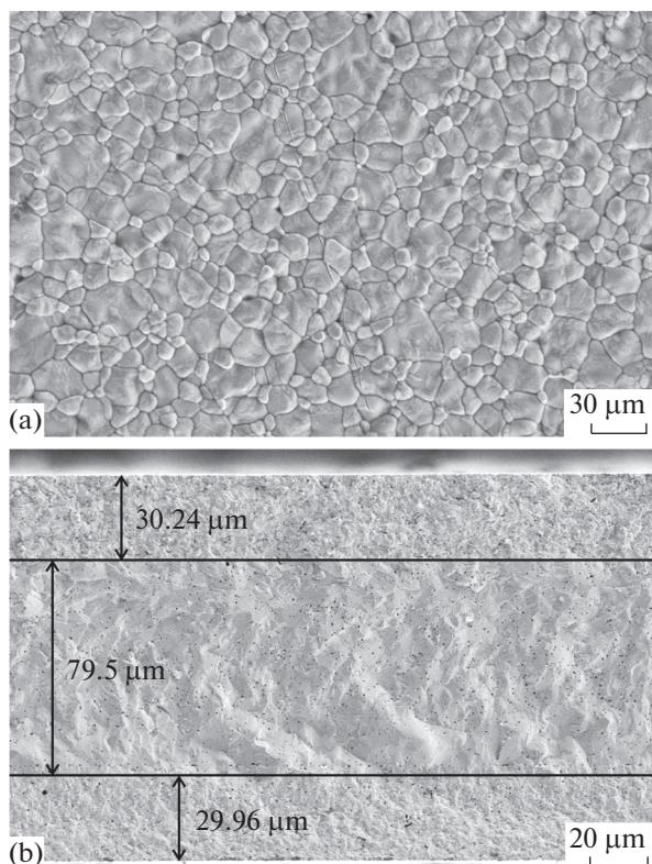
**Fig. 1.** SEM image of (a) the surface and (b) the cross-section of three-layered 6ScSZ/10Sc1YSZ/6ScSZ plates.
