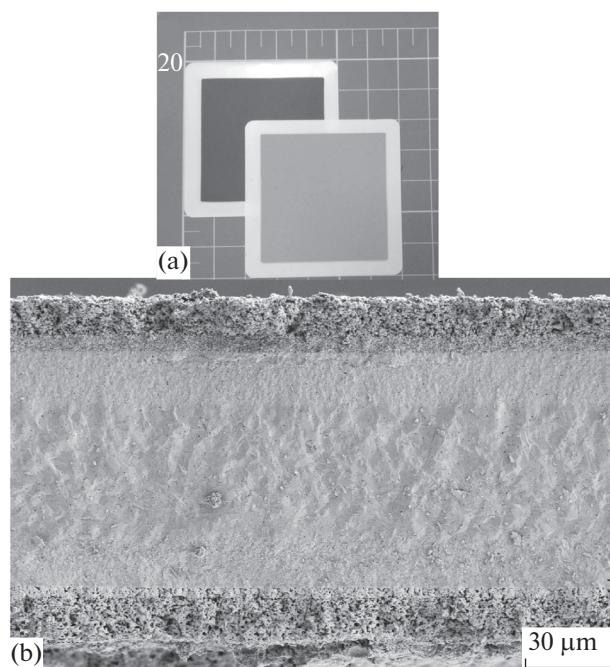
**Fig. 5.** (a) The structure of layers in multilayered ceramic membrane-electrode assemblies and (b) the SEM image of their cross-section.
