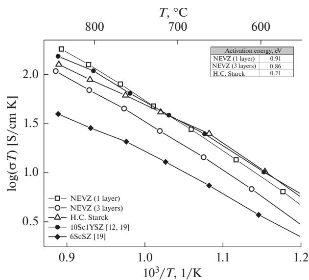
**Fig. 7.** Temperature dependence of the specific conductivity of membranes as compared with single crystals 6ScSZ and 10Sc1YSZ [12, 19].
