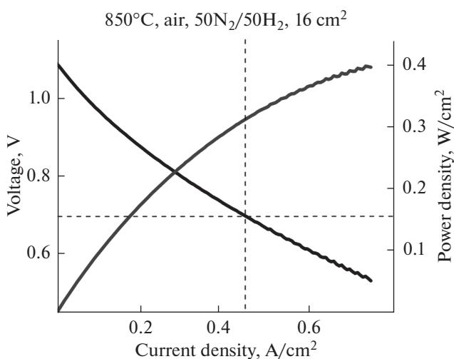
**Fig. 8.** Voltammetric and power characteristics of the membrane-electrode assembly based on three-layered membrane.
