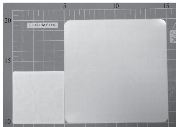
**Fig. 2.** Image of three-layered plates of the 6ScSZ/10Sc1YSZ/6ScSZ composite.
