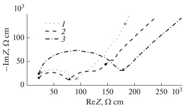
**Fig. 4.** Impedance hodographs of anionic membranes produced by (1) Stark, (2 and 3) NEVZ-Ceramics of the (2) single and (3) three-layered design measured in air at 350°C. Circles, triangles, and rhombs correspond to frequencies of 1 MHz, 10 kHz, and 100 Hz, respectively.
