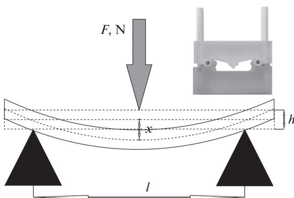
**Fig. 3.** Scheme and photograph of a sapphire setup for measuring the mechanical strength for bending of planar solid-electrolyte samples.
