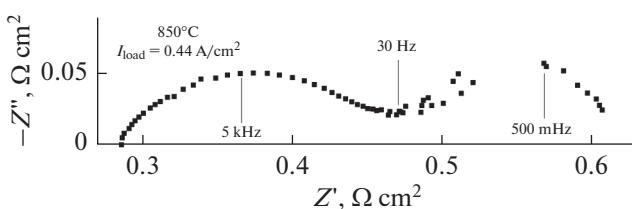
**Fig. 9.** Hodograph of impedance spectrum for membrane-electrode assembly based on three-layered membrane.
