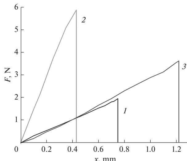
**Fig. 6.** Load curves obtained by the method of three-point bending at room temperature for (1) membrane produced by H.C. Starck and (2 and 3) single and three-layered membranes produced by NEVZ-Ceramics, respectively.
