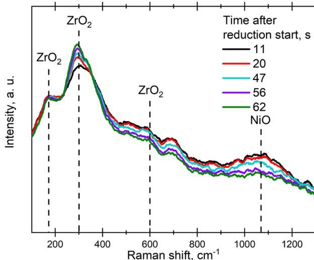
**Fig. 8** Raman spectra collected during the primary reduction of the anode-supported SOFC. Working temperature is  $600\text{ }^{\circ}\text{C}$ ; fuel gas is  $\text{H}_2$  with the flow of  $100\text{ ml/min}$ . Raman peaks around  $180$ ,  $300$ , and  $600\text{ cm}^{-1}$  correspond to lattice vibrations of zirconia in the electrolyte material, the studied NiO peak is noted in the region of  $1100\text{ cm}^{-1}$
