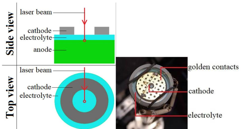
study directly the anode/electrolyte inner interface. The measuring cell, equipped with a gas mixtures supply system, was placed in a high-temperature furnace in order to ensure the operating conditions of SOFC.
