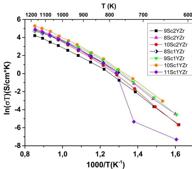
**Fig. 5.** Arrhenius plot of electrical conductivities for the  $(\text{ZrO}_2)_{1-x-y}(\text{Sc}_2\text{O}_3)_x(\text{Y}_2\text{O}_3)_y$  solid solutions crystals.
