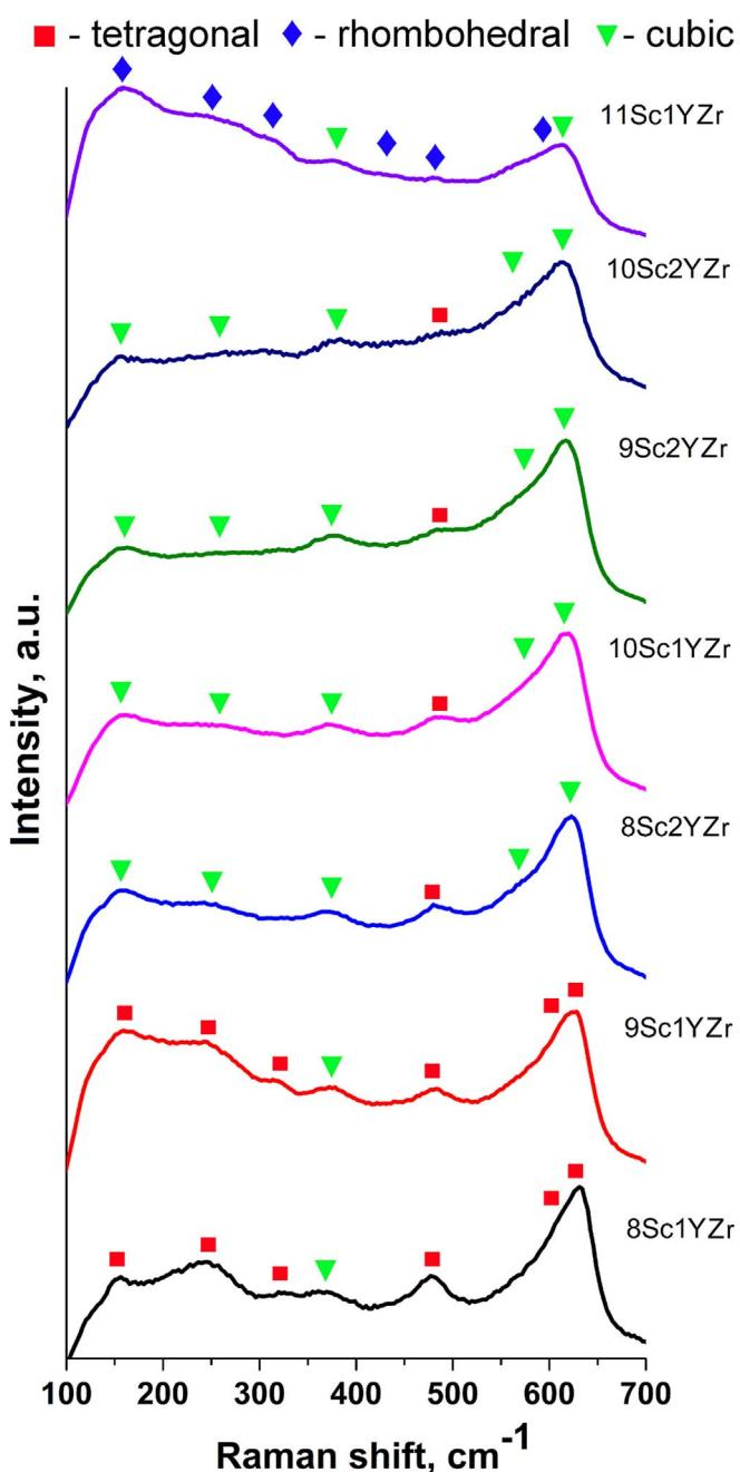
**Fig. 3.** Raman spectra of the  $(\text{ZrO}_2)_{1-x-y}(\text{Sc}_2\text{O}_3)_x(\text{Y}_2\text{O}_3)_y$  solid solution crystals. (Identification of the peaks corresponding to the tetragonal, cubic, and rhombohedral phases in accordance with [19–21]).
