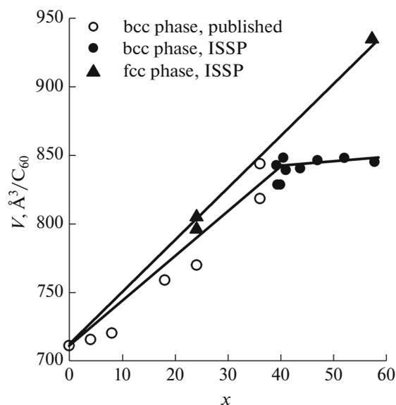
**Fig. 2.** Specific volumes  $V$  of hydrofullerites  $C_{60}H_x$  and  $C_{60}D_x$  as a function of the mean hydrogen content,  $x = H(D)/C_{60}$ .  $AlD_3$  was used to synthesize the deuterated samples. The specific volume of the hydrofullerites did not change within the experimental error with the replacement of protium with deuterium.
