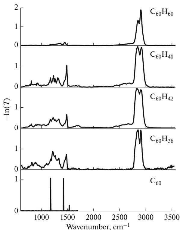
**Fig. 4.** Optical density spectra of fullerite  $C_{60}$  (normalized to unity) and hydrofullerites  $C_{60}H_x$  with  $x = 36, 42, 48,$  and  $60$  (normalized to 1.96) at  $T = 300$  K [4].
