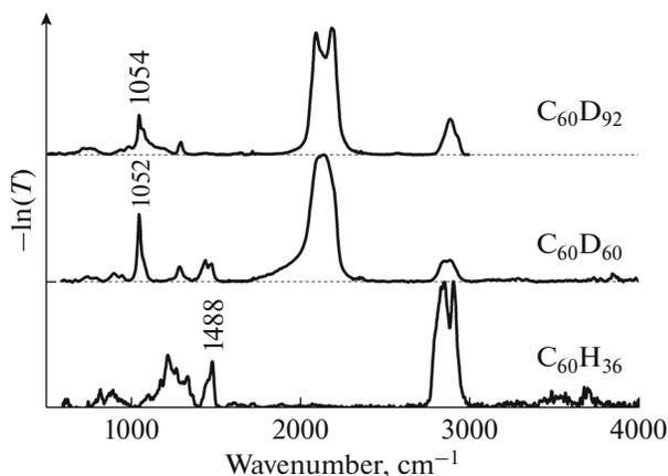
**Fig. 7.** Optical density spectra at room temperature for the crystalline hydrofullerites  $C_{60}H_{36}$  and  $C_{60}D_{60}$  with a bcc lattice and for the liquid deuterofullerite  $C_{60}D_{92}$ . The spectrum for  $C_{60}H_{36}$  is the same as in Fig. 4.
