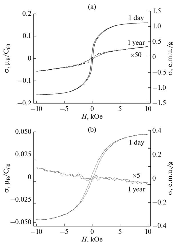
**Fig. 5.** Dependence of the magnetization  $\sigma$  on the magnetic field  $H$  at room temperature for two samples of  $C_{60}H_{24}$  with a fcc lattice and magnetization at  $H = 10$  kOe: (a)  $0.16$  and (b)  $0.046 \mu_B/C_{60}$ . The samples were synthesized at  $P_{H_2} = 0.6$  GPa and  $T = 350^\circ\text{C}$  and then kept under normal conditions for one day and one year [2].
