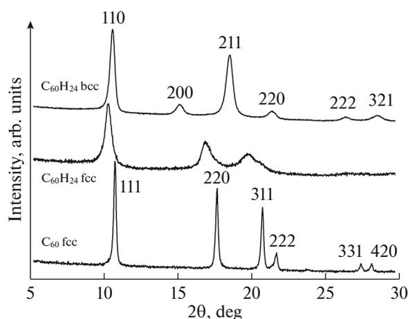
**Fig. 1.** Powder diffraction patterns of the initial fullerite  $C_{60}$  with a fcc lattice and hydrofullerites  $C_{60}H_{24}$  with fcc and bcc lattices [2]. The hydrofullerite samples were synthesized by a 24 h exposure to a hydrogen pressure of 0.6 GPa and a temperature of 350°C and, then, were kept under normal conditions for one day. The diffraction patterns were recorded at room temperature using a SIEMENS D500 diffractometer with  $CuK_{\alpha 1}$  monochromatic radiation.
